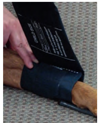
Cuff is too large. Index line won't fall within scale.
